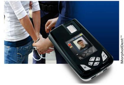
ANSI/NIST file and submits the search request to the NSP AFIS system for identification. Results are returned to the MobiLE Connexion application screen and to the MorpholDent for notification and positive identification, if available.
