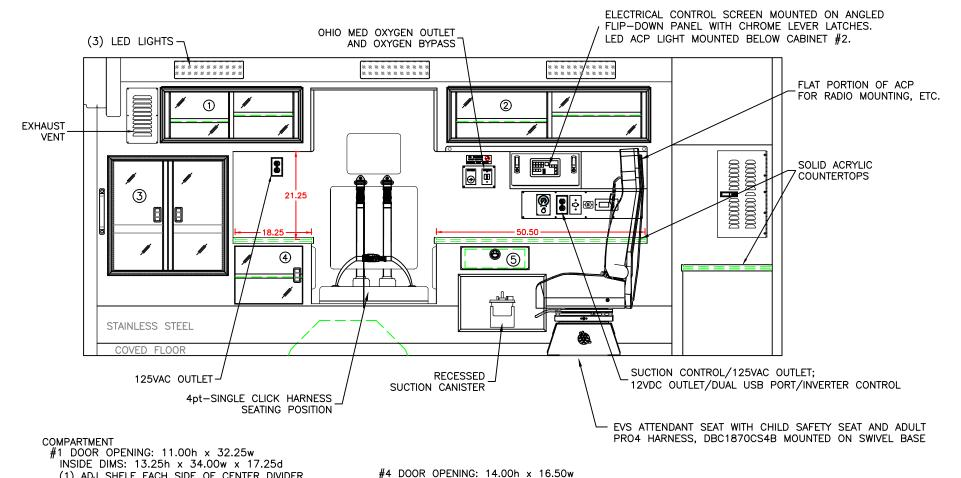
(1) ADJ SHELF EACH SIDE OF CENTER DIVIDER SLÍDING POLYCARBONATE DOORS TOTAL CABINET WEIGHT RATING = 25 lbs.
