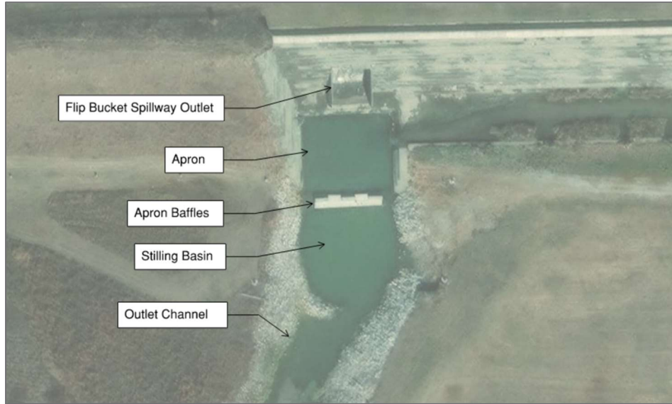
Figure 15: Principal Spillway Outlet Components
