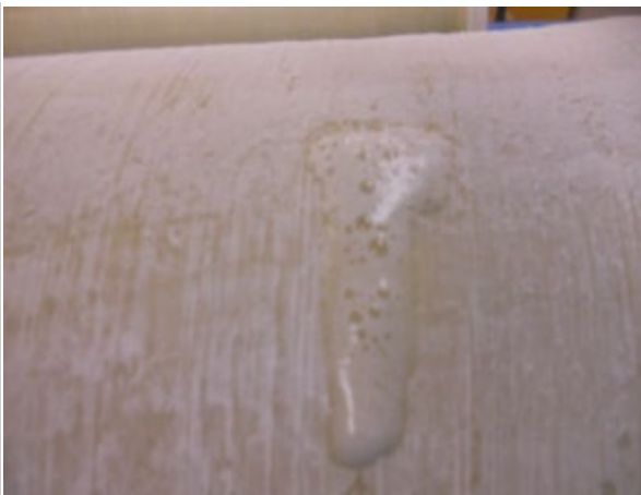
Acid reacted when applied to the foulant on the fiberglass body on J4725065
