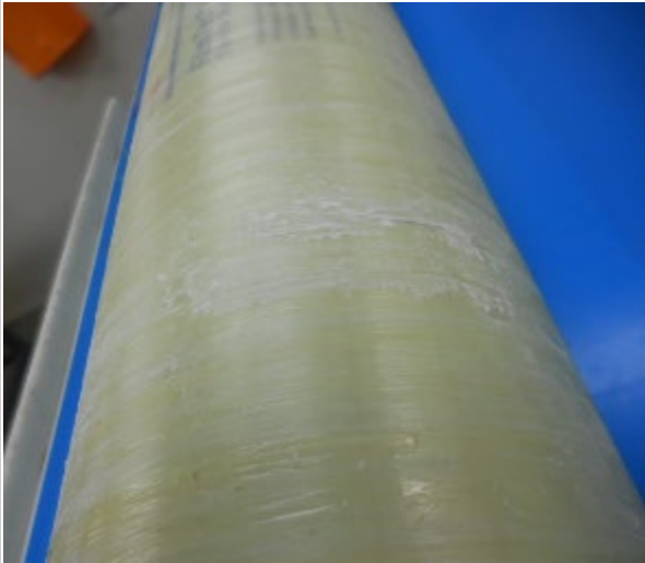
Fouled fiberglass body on J4725043
