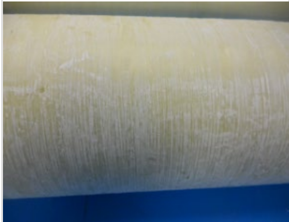
Fouled fiberglass body on J4725065
