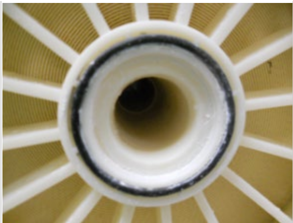
Fouled feed end PWT and o-ring on J4725065
