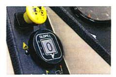
**Digital Slope Gauge**Recommended for operation on slopes.
